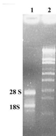
**Figure 1:** Total RNA extracted from leaves of *A. littoralis* was separated by 1% agarose gel electrophoresis and stained with ethidium bromide. 1) Total RNA extracted from sample and 2) size marker  $\lambda$ /*StyI*.
