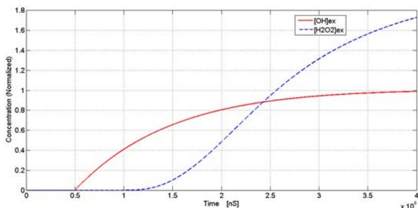
**Figure 2:** the time evolution of extracellular [OH] and [H<sub>2</sub>O<sub>2</sub>] in the bio solution. It was assumed the uniform distribution for species in the bio solution. The OH molecule is produced and its concentration increased during the discharge due to the mentioned reactions leading to generate H<sub>2</sub>O<sub>2</sub>
