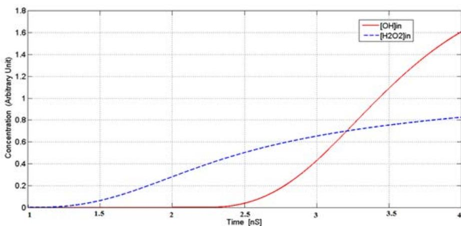
**Figure 3:** the time evolution of intracellular OH and H<sub>2</sub>O<sub>2</sub> concentrations of species which are increased due to diffusion of H<sub>2</sub>O<sub>2</sub> toward the inside of cell.
