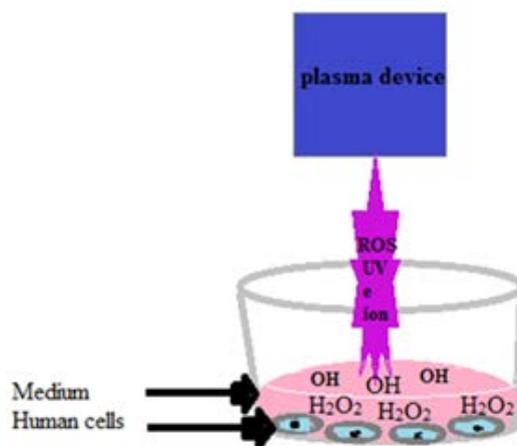
**Figure 1:** Schematic illustration for the interaction between NTP and cells *in vitro*. The reactive species formations in the culture medium (particularly hydroxyl) have been regarded as the main factors causing the death of cancer cells *in vitro*.
